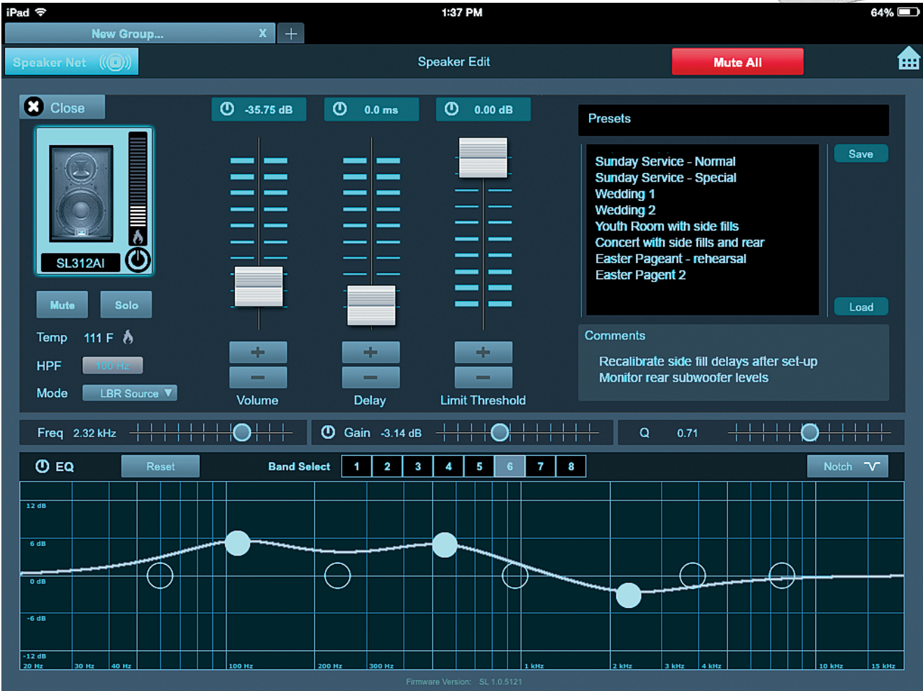
The Speaker Edit page lets you set EQ and alignment delay, add notch filters, and remote-control onboard speaker settings.
