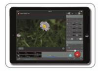
The Zebra filter uses striped patterns to indicate the overexposed and/or underexposed areas of the image.
