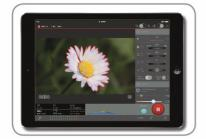
The Focus Peaking Filter highlights the focused profiles (intesity and color profile can be adjusted) on the image.
