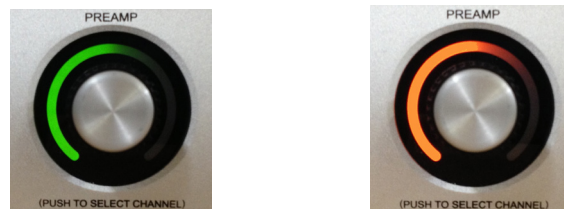
Apollo's front panel preamp knob during normal operation (left) and when a Unison plug-in is inserted in Console's INPUT insert slot of Apollo's selected channel (right)
