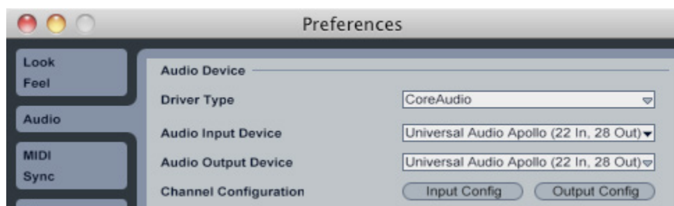
Apollo selected as the Core Audio I/O device in Ableton Live preferences
