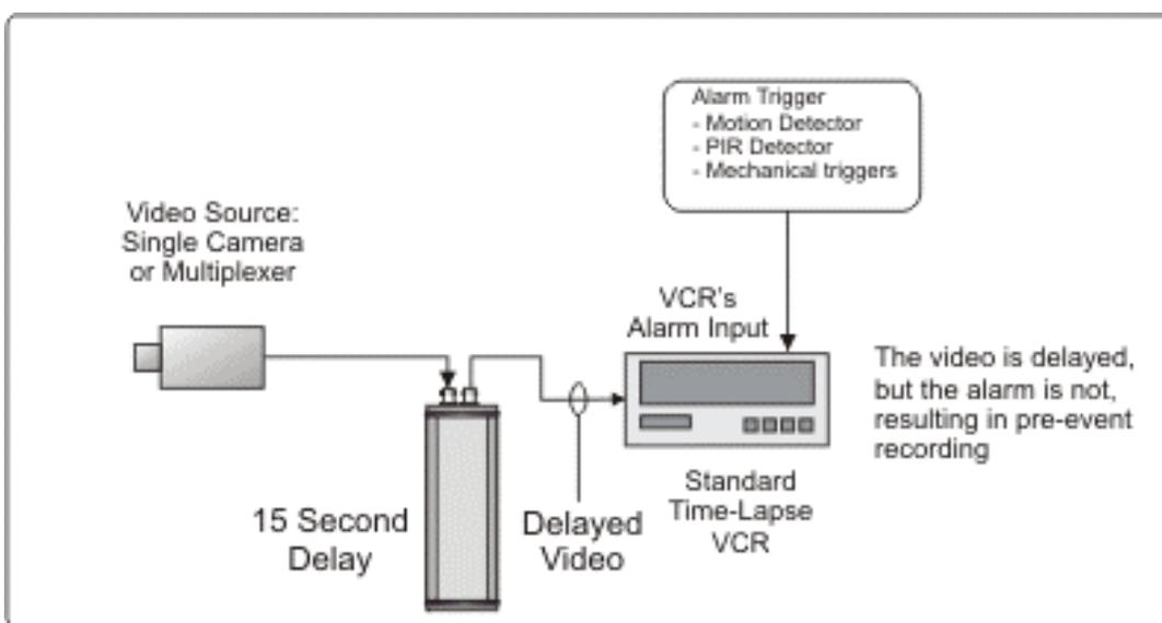
DelaySystem can be used to upgrade a standard time-lapse VCR to pre-event recording. This is an advanced feature, which is normally associated with digital
