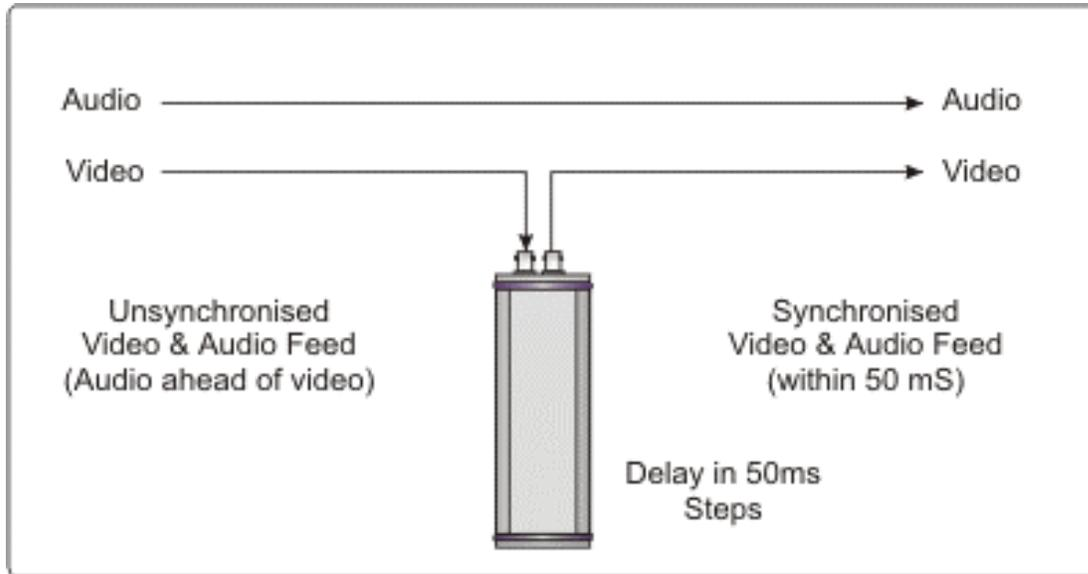
Digital video and audio compression and transmission systems can introduce differing amounts of delay to video and audio signals. “Lip-Sync” requires video and audio synchronization otherwise the viewer becomes distracted by the lack of coordination between the subject’s lips and voice. If the audio is delayed more than the video, DelaySystem can be used to synchronize the two feeds.
