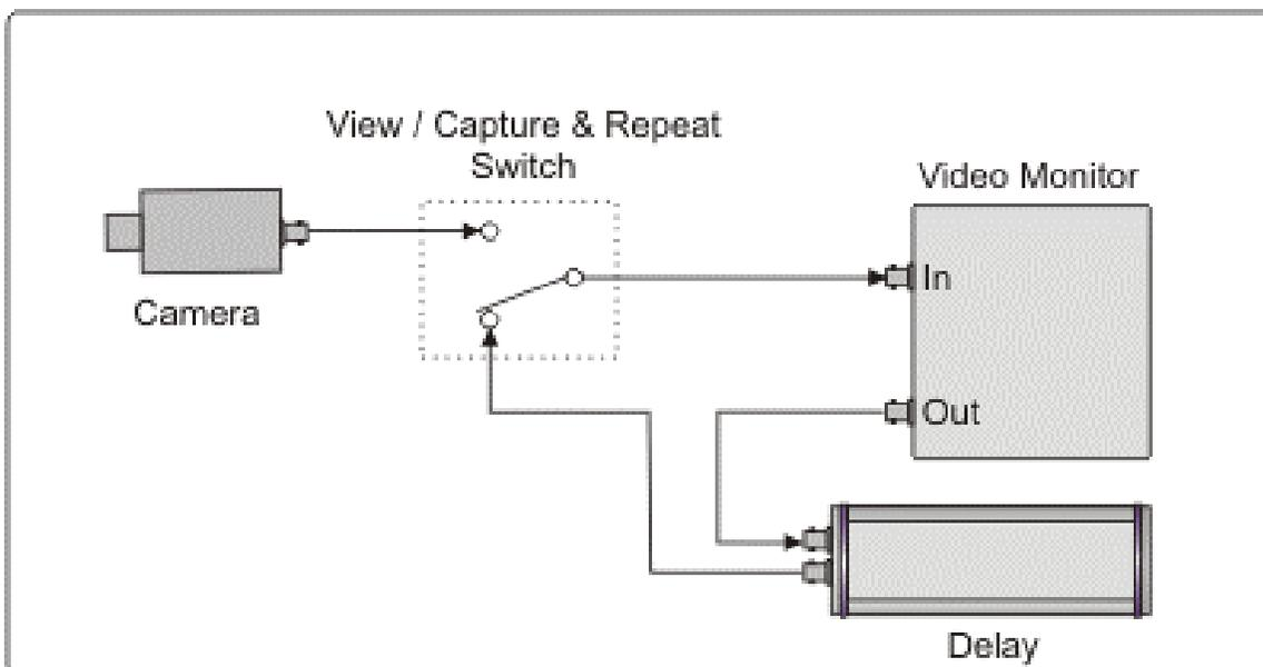
With an external video switch and monitor, DelaySystem can be used to capture an event and constantly repeat it. With the switch in the normal "view" position the operator sees the live video. If an event of interest occurs, the operator may switch over to the delayed version, which will replay the event (of say 10 seconds duration) and then constantly repeat the event as it is fed back into the DelaySystem.
