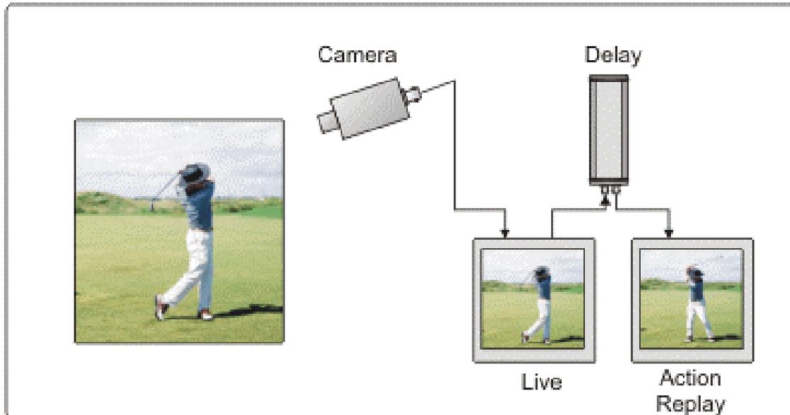
DelaySystem video delay line temporarily stores up to 2 minutes of video. It is therefore possible to use the delay line to replay an event of interest without the need to stop and rewind a video recorder. For example, a CCTV operator can double-check if an offence has taken place by switching to the delayed video, which will replay the event a few seconds later.
