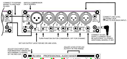
IF COMPRESSOR IS TURNED ON, LED TFLASHES WHEN COMPRESSOR IS ACTIVE
