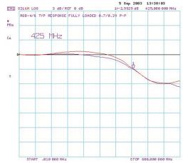
The above graph illustrates the typical frequency response of the RGB - 4/6. Notice that the cuves represent a fully loaded unit and show the response to a 0.7V p-p and a 0.2V p-p input signals. It is important to observe that the overal flatness and upper limits are fairly independent of signal amplitude. This is an extremely important characteristic.
