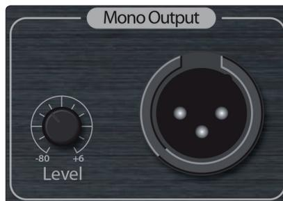
The XLR jacks are electrically balanced and rated +24 dBu maximum output level. They are wired as follows:
