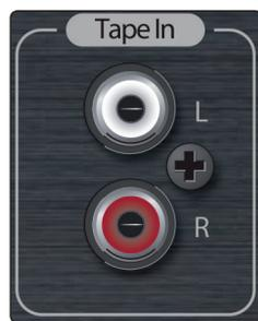
The Tape In connections on the front panel are RCA jacks that accept consumer line-level signals (-10 dBV nominal). These inputs can be used for playback from CD players, MP3 players, and other consumer devices. In UC Surface, these inputs show up as a stereo tape return channel strip. For more information, *see Chapter 4, "UC Surface," in the StudioLive-AI Software Library Manual.*
