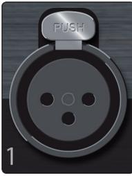
Your StudioLive RM-series mixer is equipped with 32/16 recallable PreSonus XMAX microphone preamplifiers for use with all types of microphones. The XMAX preamplifier has a Class A input buffer allowing you to boost signals without increasing unwanted background noise.
