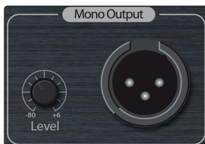
The Mono/Center output carries the Mono or Center mix and is convenient for feeding mono sound systems, such as a center channel send for true LCR mixing or a subwoofer send. Signals are assigned to the Mono mix in the UC Surface mixer.
