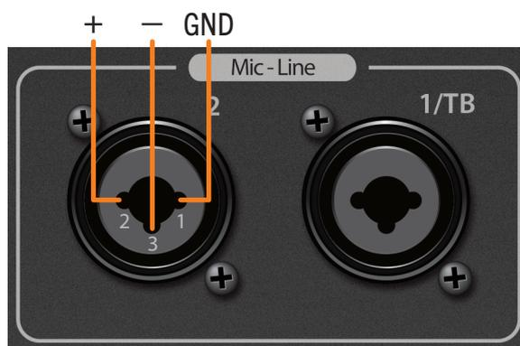
Pin 1 = GND; Pin 2 = Signal +; Pin 3 = Signal -
