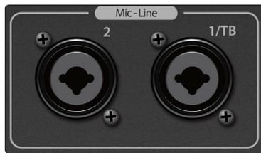
7. **Mic/Line Inputs.** These XLR-TRS combo jacks feed the microphone and line inputs for the control surface. The XLR feeds through a recallable XMAX preamp. The TRS input feeds the line-level input and bypasses the preamp with a fixed signal to the analog-to-digital converter.
