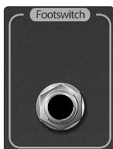
6. **Footswitch Input.** A 1/4-inch jack supports a momentary footswitch. The target for footswitch control is set in the Master Control touchscreen.
