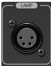
3. **Lamp Jack.** The 4-pin XLR lamp jack provides 12 volts to support high-intensity lamps.
