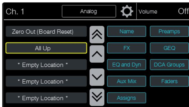
Quick Recall eliminates the step of pressing the Recall button, which is faster than explicitly pressing the button but more vulnerable to accidental scene loading. It is useful any time you think you may need to switch mix scenes quickly.
