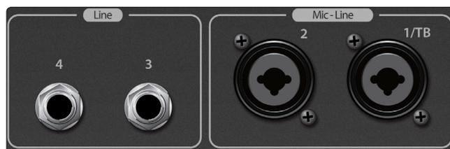
The microphone inputs on the CS18AI utilize the same recallable XMAX preamps as RM-series mixers, ensuring you have high-quality audio that's sonically matched with your mixer.
