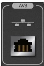
5. **Ethernet AVB Jack.** This RJ-45 jack supports Ethernet AVB networking, with integrated connection and activity indicators. It provides the primary control and audio transport. When connected on an AVB-compliant network or to an AVB-compliant device, the built-in 4x2 audio is available on the network. When connected to a non-AVB-compliant network or device, only control data is available.
