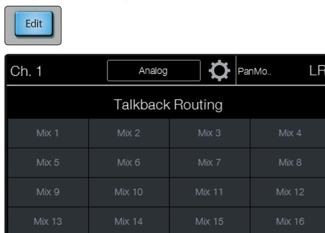
At the top of the Talkback Assign screen you can see the current talkback input source and a gear icon. Pressing the gear icon brings you to the Talkback Settings screen. Here you can select a different talkback source, adjust the talkback preamp level, and engage +48 phantom power on the talkback input.
