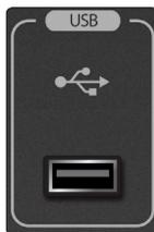
4. **USB Port.** The USB Type-A port is used for firmware updates using a thumb drive and for Wi-Fi connections using the included USB Wi-Fi LAN adapter.
