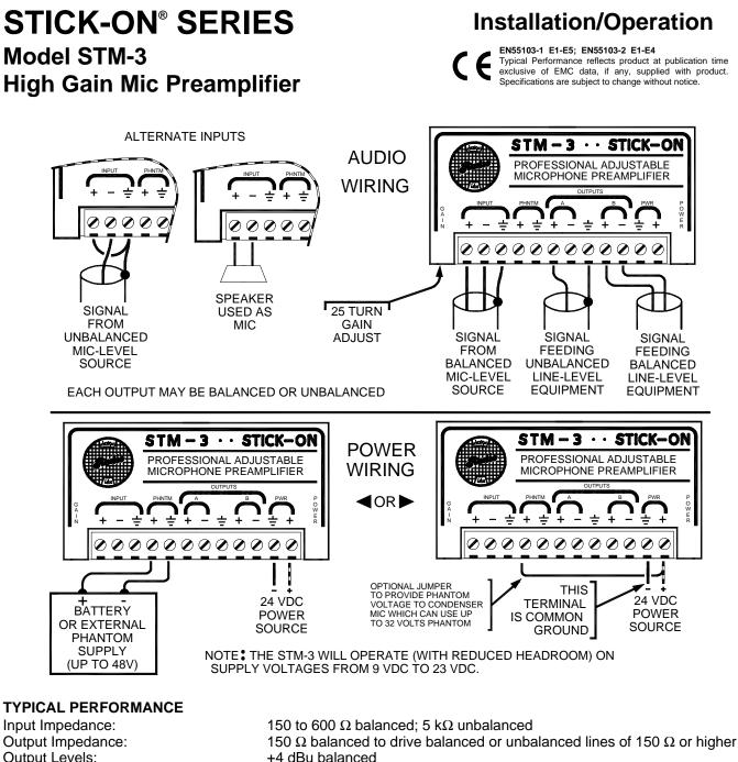
Output Impedance. Output Levels: Frequency Response: Gain: THD+N: CMRR: Headroom: Power Requirement:
