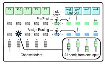
Press an Input Channel strip Mix key.
