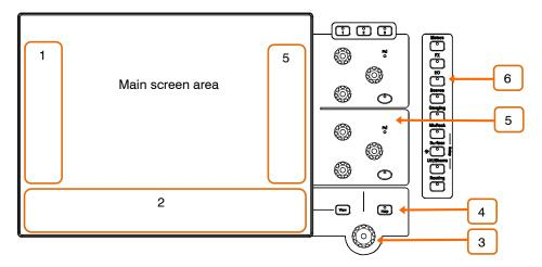
Left widget area – Can be configured for different functions, for example as a scrollable Scenes list. Hold down **Setup** and touch this area to configure.
