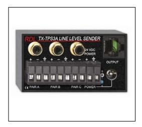
The TX-TPS3A is a three-pair audio sending module compatible with RDL Format-A twisted pair products. It is built in the versatile Max-TX series enclosure. The durable adhesives provided with the TX-TPS3A permit permanent or removable mounting. The TX-TPS3A may be rack or surface mounted with optional TX<sup>™</sup> series accessories.
