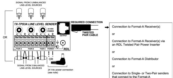
NOTE: Connect a 24 Vdc power supply to the module if power is not being supplied through a twisted pair cable from a connected module.
