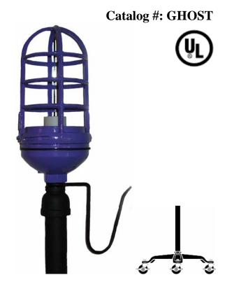
The Behind the Scenes Ghostlight comes with the protective basket and base assembly finished in Behind the Scenes Purple. The stand and locking three-wheeled base are finished in black enamel. The unit is furnished with a 15′ 12/3 SJ cable with a parallel blade and ground connector; cable hook; and a medium screw-base socket. The unit is UL-Listed as a Portable Luminaire, Issue BK 09976 and is rated for a 100-Amp maximum Type A lamp.
