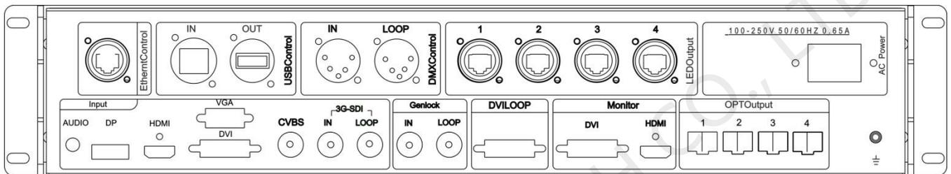
Ethernet: Internet port can be connected with PC for communication through standard TCP/IP protocol.
