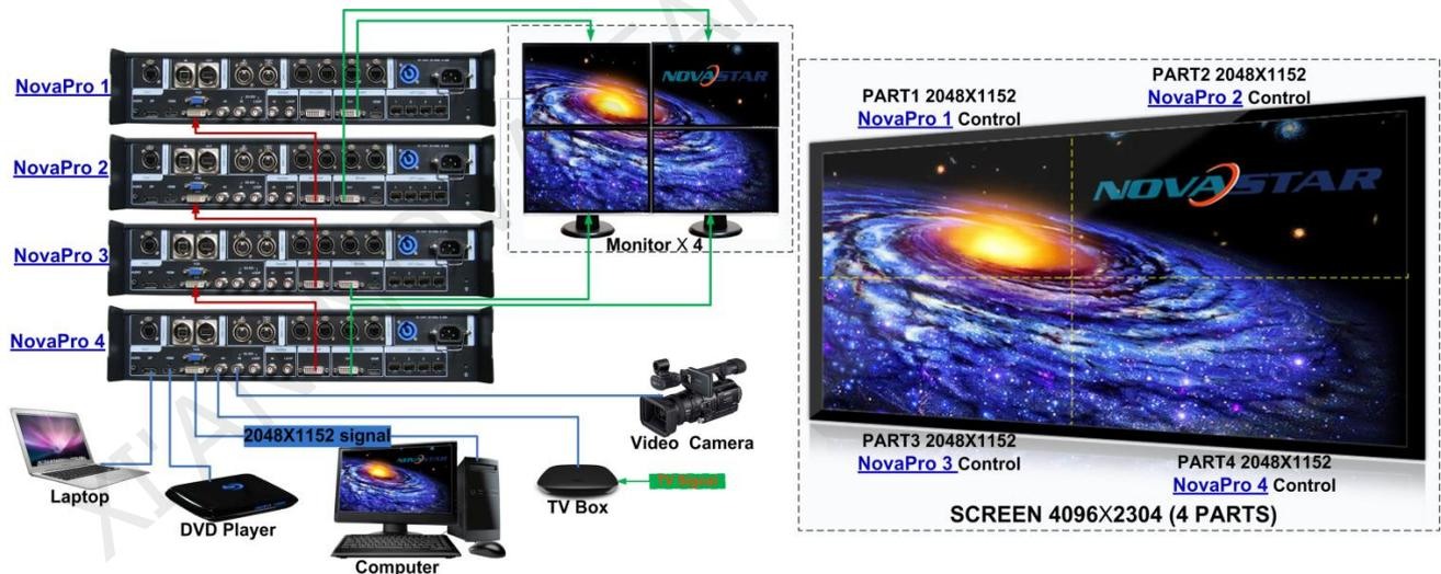
Fig. 4-1 4K Resolution large load-carrying scheme
