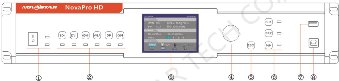
①: Red indicating light corresponds to power switch and green light corresponds to working state indicating light. When it works normally, green light normally blinks. When there is no video input signal, blinking is slow. When any internet port is in hot backup state in this equipment, breathing blinking is shown.
