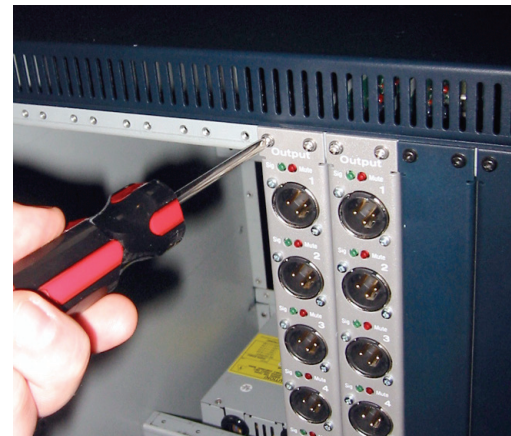
Securing a Stage Rack option card to the Stage Rack front panel
