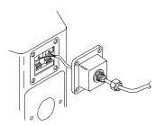
Step 4 – Remove the protective paper over the adhesive gasket surrounding the underside of the MTC-PC2. Attach MTC-PC2 through the existing screw holes, USING THE SCREWS PROVIDED WITH THE MTC-PC2. It might be necessary, depending on the stiffness of the cable, to slide the cable through the gland fitting to avoid strain on the wire or connections inside the panel cover.
