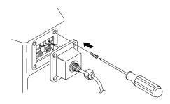
Step 5 – Tighten the nut on the gland fitting to seal around the cable to a recommended torque of 80 in lbs. The fitting is specified to be liquid-tight for round cables and many off-round cables. If the fitting does not achieve a tight seal on a particular cable type, it might be necessary to use a different, rounder, cable type..
