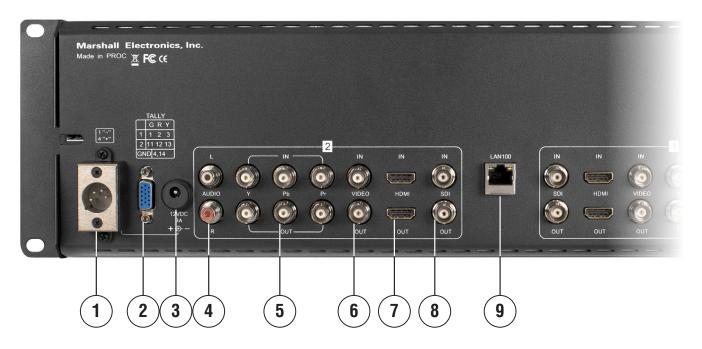
Note: Each screen has its own full complement of video input connections. Power, TALLY and LAN connections go to both screens
