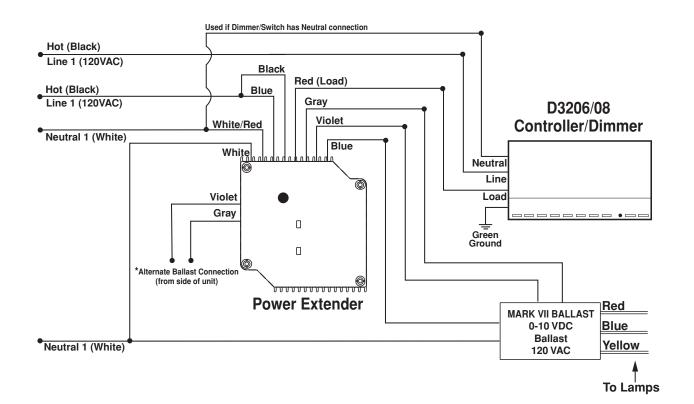
Wiring Diagram 1B - Power Supply connected to Load side, 120V Application
