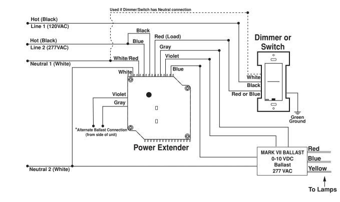
NOTE: In 277V applications, the dimmer or switch must still be wired for 120V.
