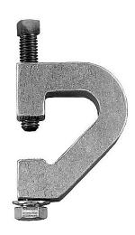
The Purlin Clamp is perfect for installing to purlins, I-beams and bar joists up to I" thick.  $I/2'' \times 2.5''$  square head set screw for locking onto I-beam.  $I/2'' \times I''$  grade 5 Hex Head Bolt supplied to connect load or use for I/2'' - I3 tpi threaded rod. Micro-grooves for secure connection to beam. I" thick.
