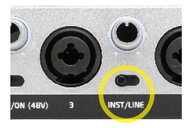
Note that the setting of the INST/LINE switch affects input monitoring even when only microphones are connected to the T4. In this case, set the INST/LINE switch for each pair to LINE if you want to monitor the incoming mic signal(s) in stereo, or to INST if you want to monitor in mono.
