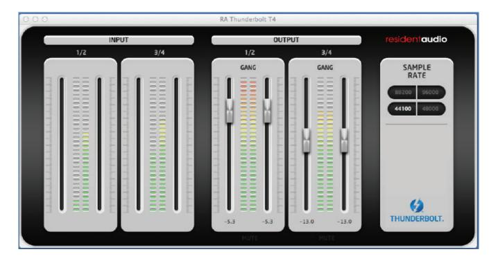
When a connection is made to Output jack 4 (thereby placing the T4 in Multichannel Mode), all four output level sliders in the Digital Panel go to the 0 position and all sound is muted (the Big Knob control affect headphone level only). To set the sound to the desired levels, simply "grab" and move each slider with your mouse.
