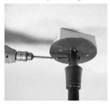
Insert bolt thru hole and put nut for security.
