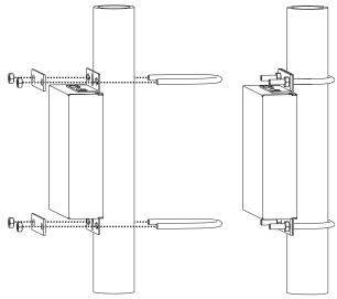
FIG. 9 Mount to projector pipe with bolts through brackets
