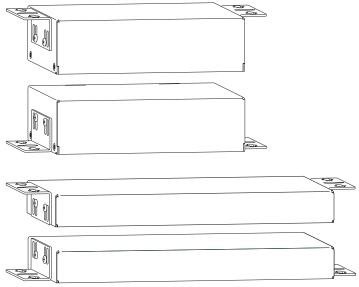
FIG. 3 Attach brackets in either top or bottom position (various size modules shown)
