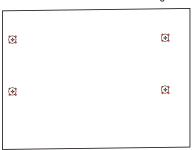
FIG. 6 Drill pilot holes and start screws, but do not tighten
