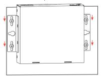
FIG. 7 Align module over screws and slide into place
