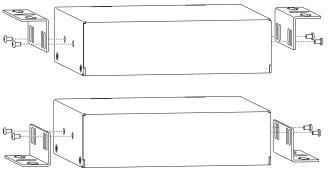
FIG. 4 Insert screws and tighten
