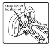
screw and securely fasten mounting plate to surface (user must supply fasteners). Mounting bracket may also be strap-mounted to pole or appropriate anchor point.
