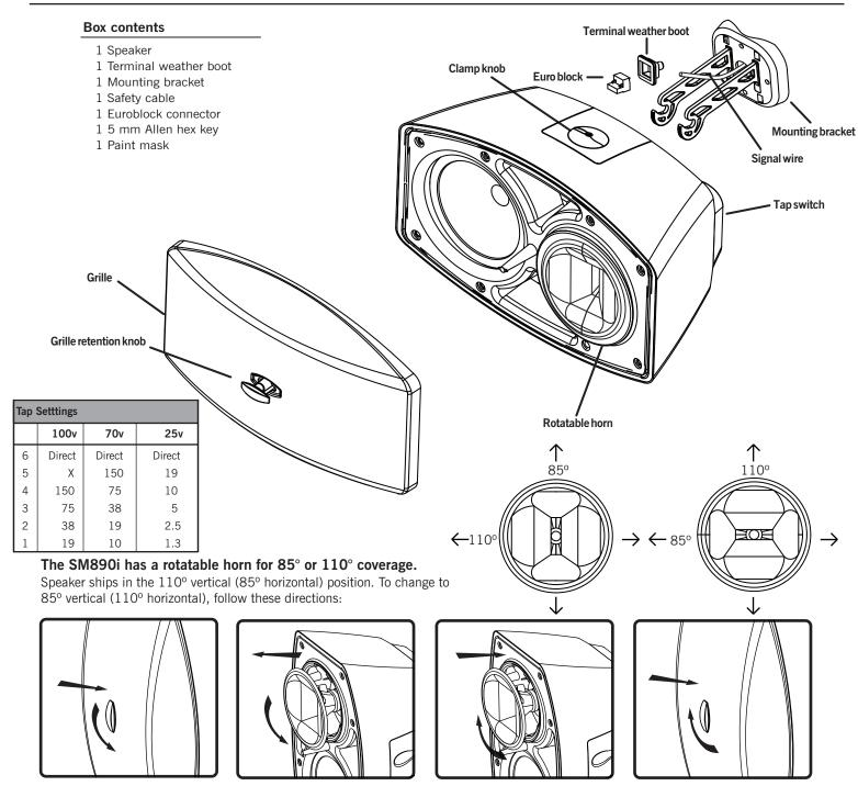
**1.** To remove the grille, rotate the grille retention knob counter-clockwise while gently pushing down on the grille. Remove the grille from the speaker by pulling gently on the grille retention knob.
