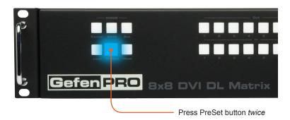
2 Press an Input button (1 - 8) to store the current routing state.
