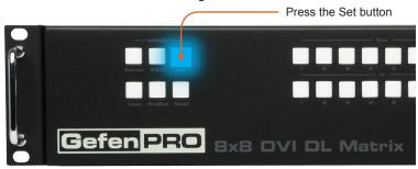
2 Press any Input on the bottom row of buttons (1 - 8). The system indicates the current routing status.
