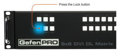
2 Press the Lock button a second time to deactivate System Lock Mode.
