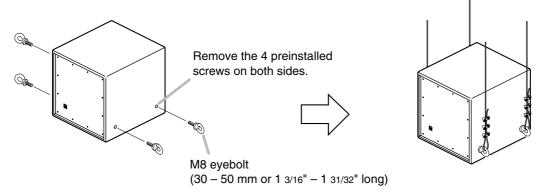
Use the optional HY-PF1B or HY-PF1W Speaker Rigging Frame to suspend the FB-120 subwoofer together in the same location with TOA HX-5 series speakers.
