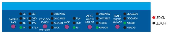
In this mode both the AD and DA run on the internal clock. This mode provides the lowest jitter and most sonically robust performance. External recorders (such as DAW etc) have to be synchronized either to the AD digital outputs (any format: AES or DIOCARD1 or DIOCARD2) or to the converter Worclock output.
