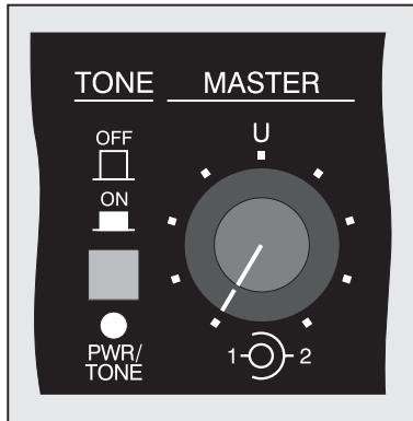
Figure 9. Detail of front panel showing the power/tone LED indicator
