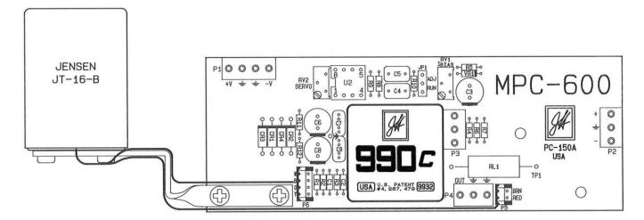
The MPC-600 mic preamp card dramatically improves the performance of MCI 600-series consoles. The combination of the Jensen JT-16-B mic-input transformer (Jensen's best mic-input model), the 990C discrete class-A op-amp, and the total absence of coupling capacitors in the signal path results in superior audio performance. Just plug it in!
