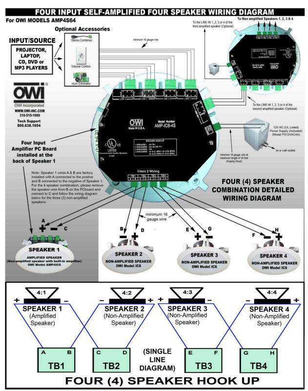
Filename: AMP4IC6 4 Input Detailed Wiring Diagram 4 SPEAKER 10/25/12
