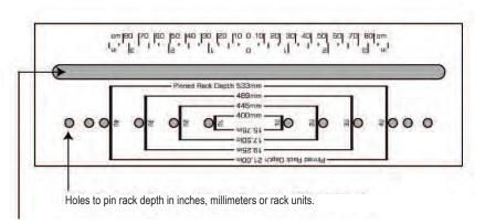
Slot to set rack depth in alternate sizes.
