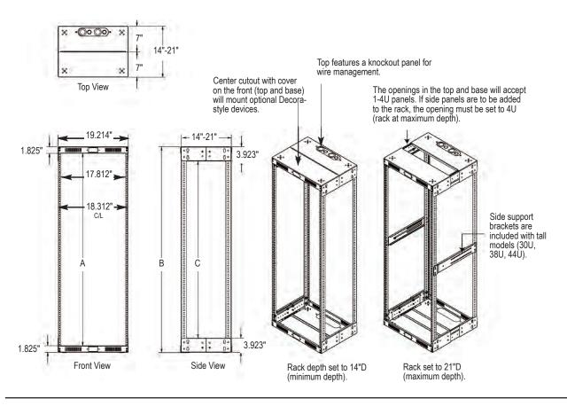
**Optional Side Panels:** Side panels extend 1" beyond rack (.5" front, .5" rear). Each side panel is .625" thick; two side panels will increase overall rack width from 19.214" to 20.5".
