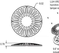
LUH-VRG mounts to the horn/trim ring using tamper-resistant screws
