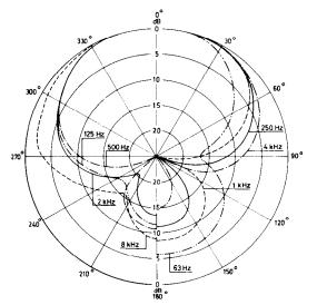
This polar pattern and frequency response curve correspond to typical machine run specifications from a standard M 160.
