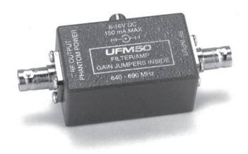
The UFM50 provides a unique, high performance solution for antenna systems requiring long cable runs or distribution to multiple receivers or locations. The unit can be used to apply RF gain at the antenna ahead of a long run of coaxial cable to compensate for signal loss through the cable. A compact, high performance multicoupler can also be configured using the UFM50 ahead of an RF splitter to offset the loss through the splitter.
