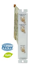
The LV 58SER03 provides the LV 5800 with two composite (NTSC/ PAL) inputs. The LV 5800's newest functions related to waveforms such as the waveform monitor, vectorscope, and simple picture monitor can be used on analog video signals of NTSC and PAL formats.
