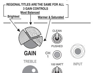
each channel looks identical, the **GAIN** Control for each channel comes in a different place and adjusts a different point in that channels circuit.
