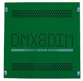
The dmx8dim is an eight output 'green' dimmer designed for high efficacy loads, low idle power, and minimal losses. Typical loads include LED lamps, Neon, Compact Fluorescent, Electronic and Magnetic Low Voltage, and low power halogen.
