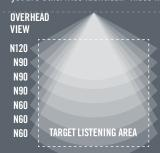
matched", within the same line array column, allowing designers to reap the benefits of a line array solution, while retaining the ability to configure horizontal coverage. This simple illustration shows how seven IN.LINETM modules could completely cover a rectangular listening space, while keeping excess acoustic energy off the walls.
