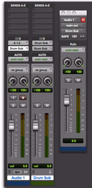
New Auxiliary Input track with audio track send automatically assigned to an internal mix bus named “Drum Sub”
