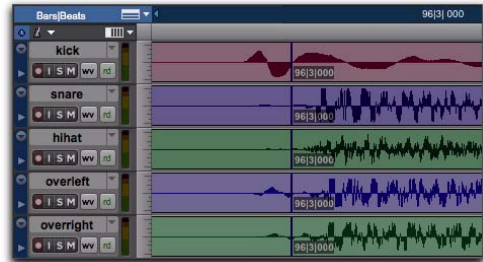
Figure 5. Overhead mics generate late beat triggers
