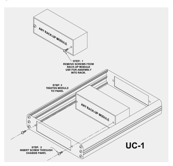
Install Rack-Up modules in the front or rear openings using the spacers provided. Orient the spacers as shown in the diagram. Spacers are not required when mounting RDL AMS accessories. UC-1 chassis is shown with top cover removed.
