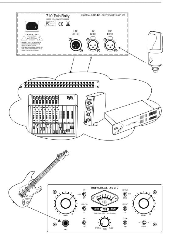
For most applications, we recommend setting the 710 Gain and Level controls at approximately "5" (their twelve o'clock position). Adjustments can then be made to the Gain, Level, and Blend controls to achieve the optimum sound for your signal source.
