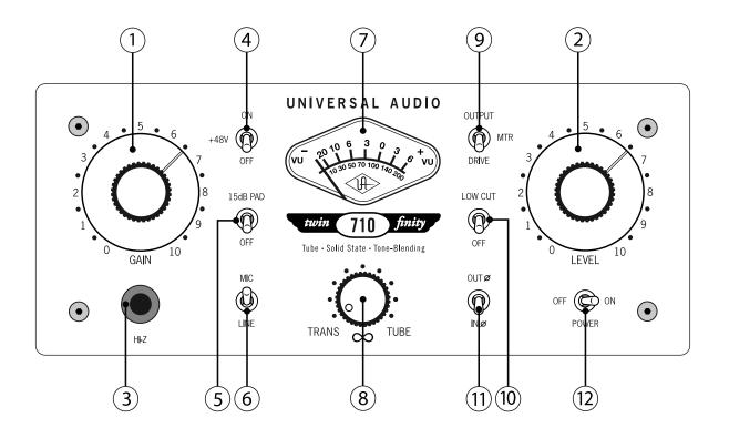
(1) **Gain** - Adjusts the gain of the input stage. Turning this knob clockwise raises the amount of gain applied to the input signal.
